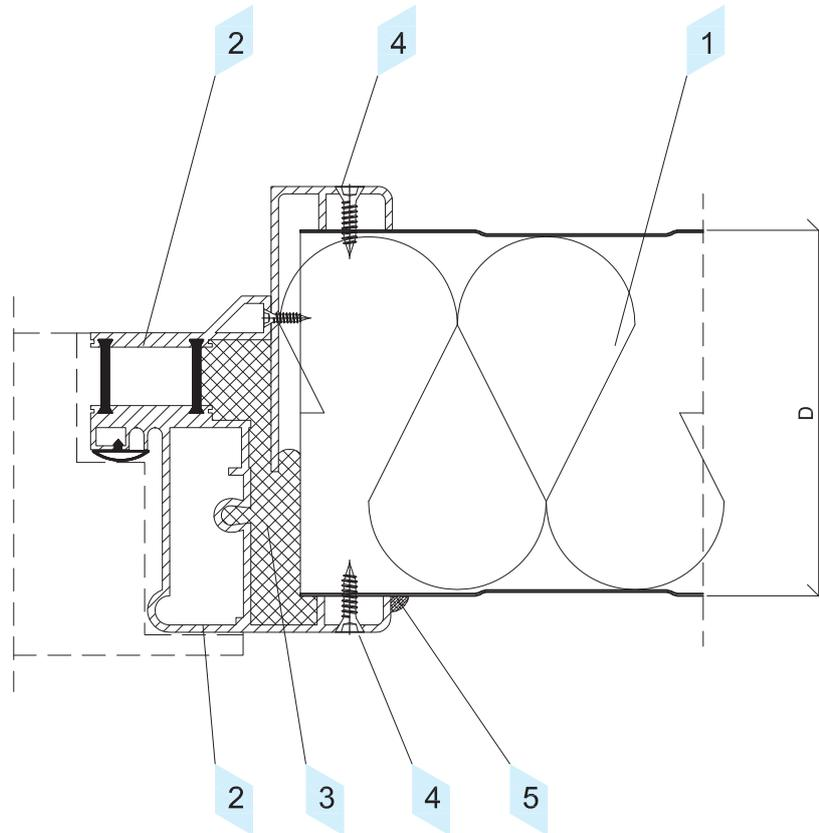
**4.16 Jointing of the external wall with the door frame detail**
